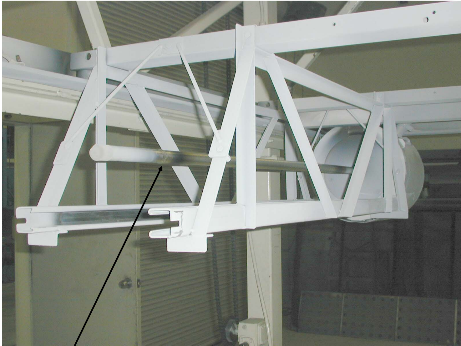
Long Aluminum Sputter Probe on IVD Rack
