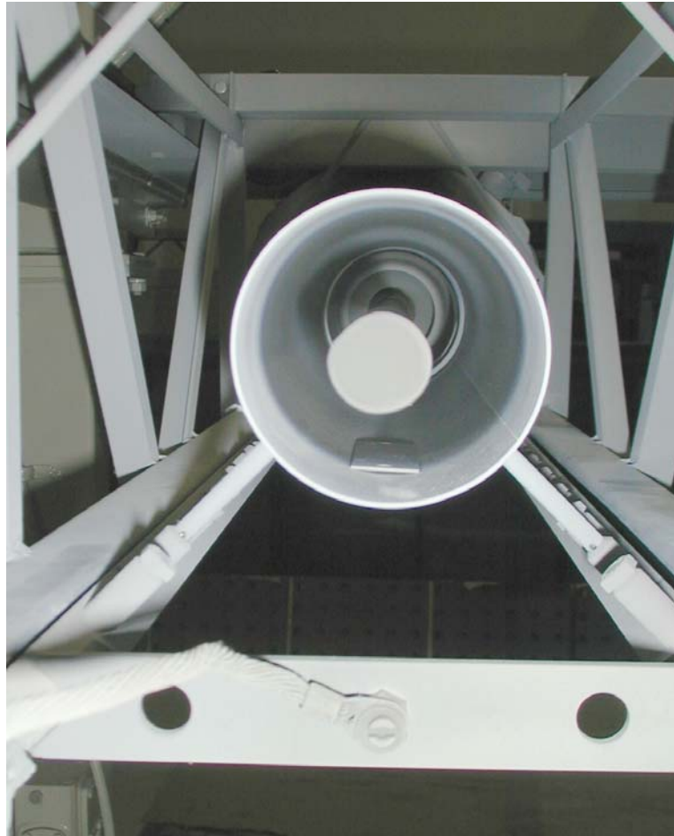
Sputter Probe Aligned In Center of Part
