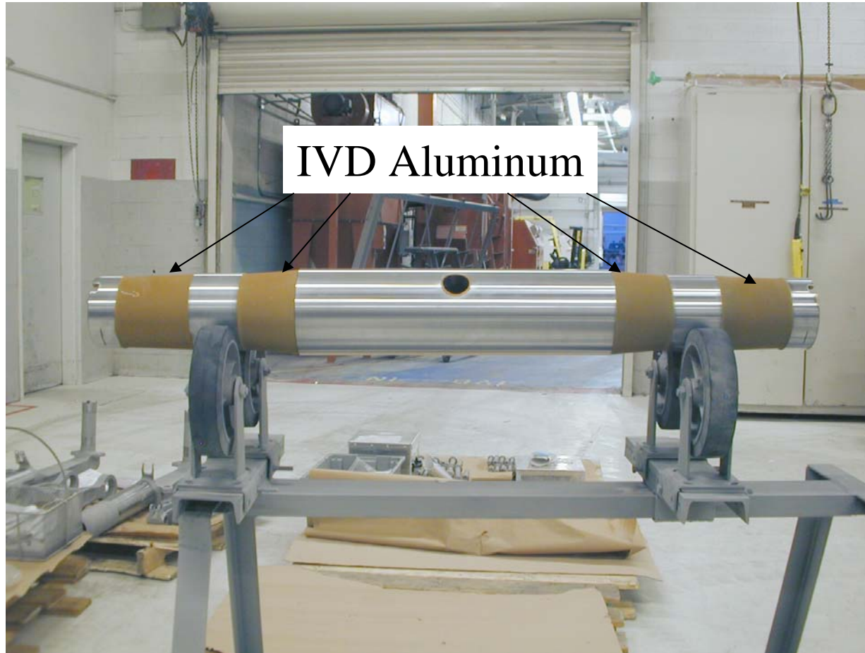
C-17 Axle After Conversion Coating
