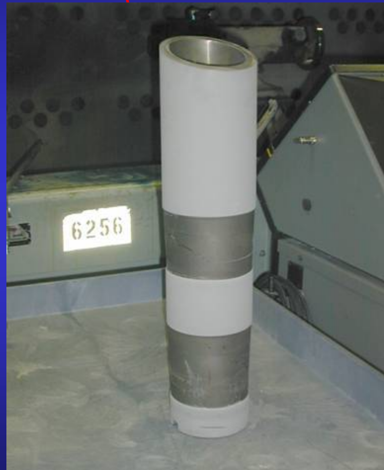
Hill AFB HVOF Coating C-17 MLG Wheel Axle
