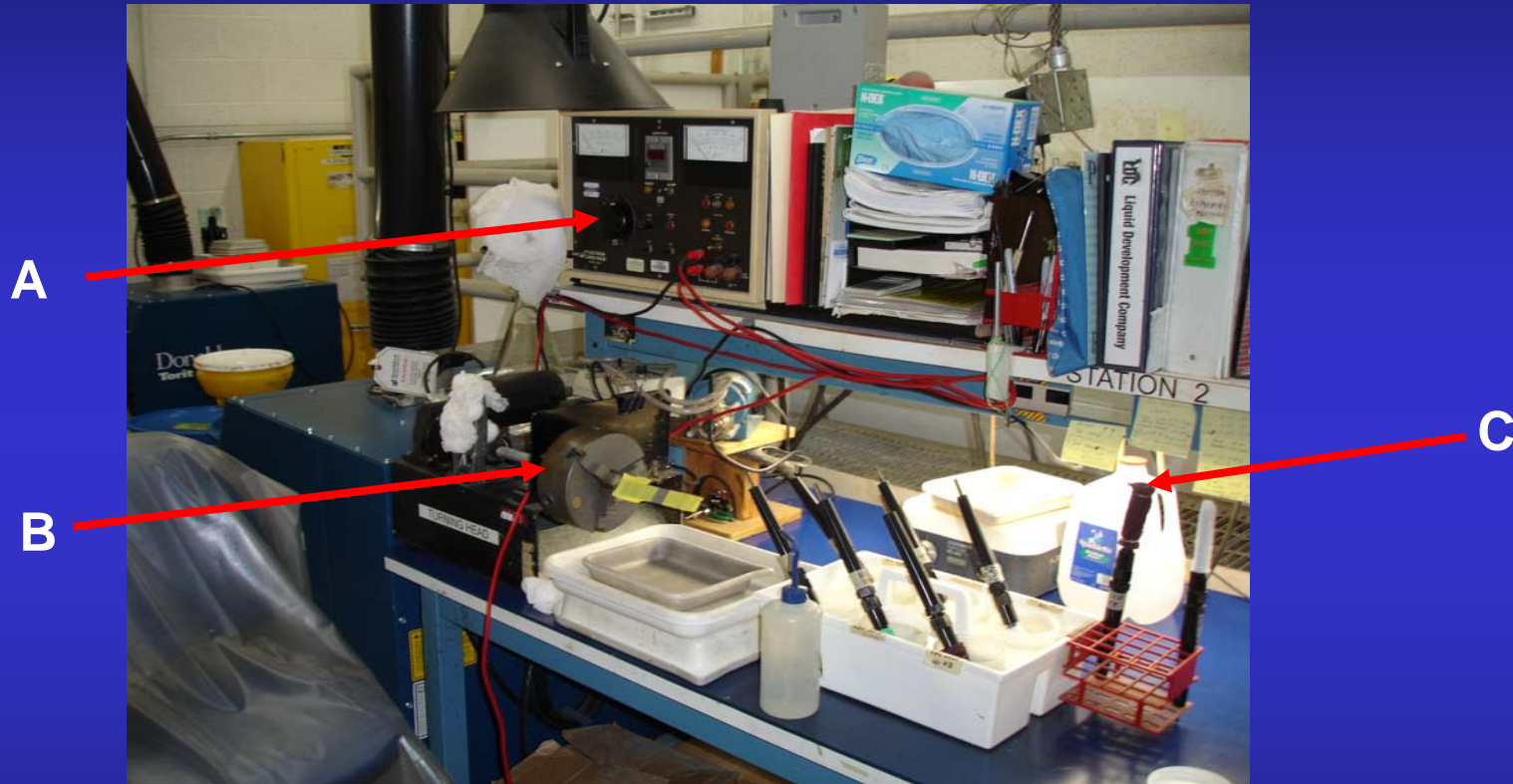
Brush Plate Flow Process with D.C. Power Supply (A), Panel Holder (B) and Brush Plate Tool/Anode (C).
