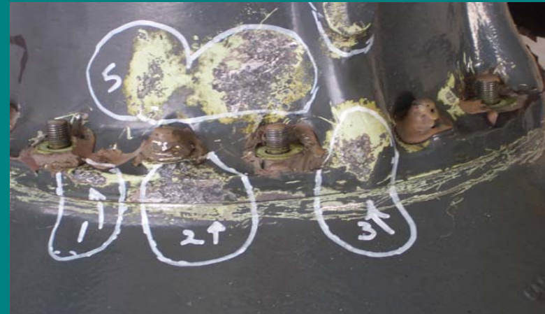
H-60 Main Transmission Housing showing areas most susceptible to corrosion
