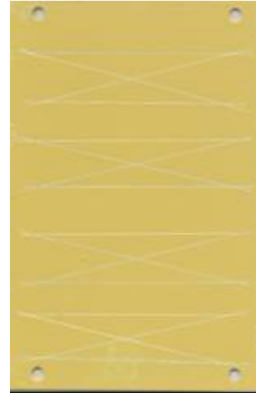
Electroplated Al with MIL-PRF- 23377, after 7 days
