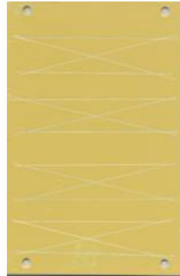
Electroplated Al with MIL-PRF- 23377, after 7 days
