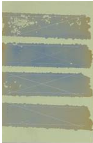
LHE Zn-Ni with MIL-PRF-85582 C1, after 4 days
