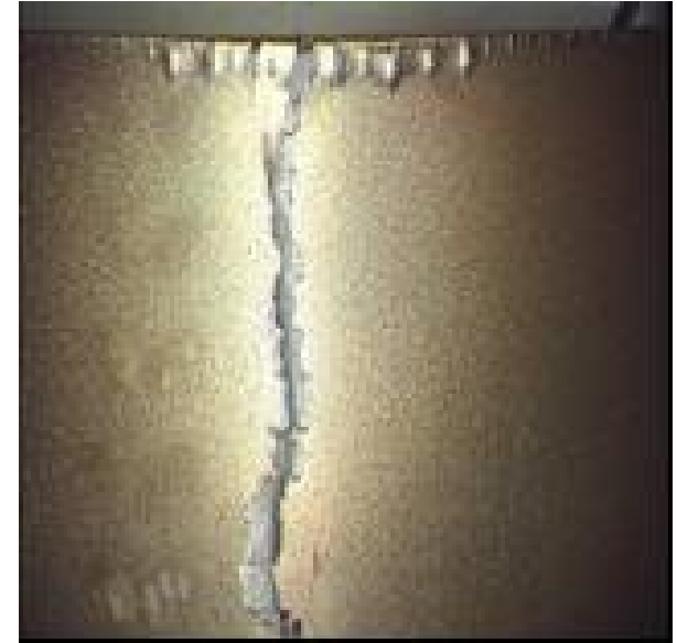
Electroplated Aluminum on Ti-6-4
