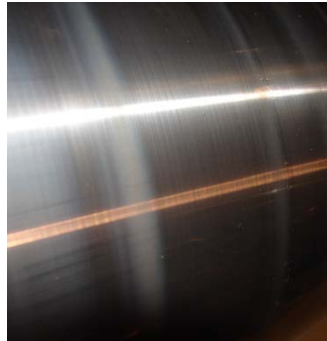
Finish shows circumferential finish profile and "polishing" affect of the bearing interaction (roughly 3,500 Landing Sequences)
