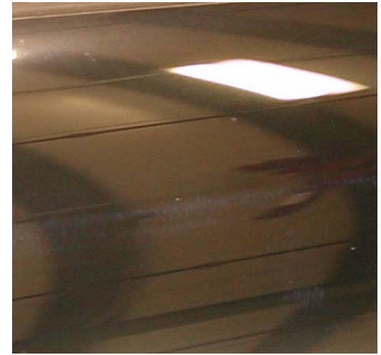
Large HVOF Slider (After 21,550 Landing Sequences) Shows the reflection of the overhead in the lab ceiling – no visible dynamic affects from testing
